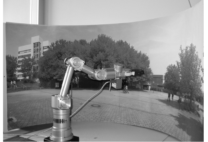
Fig. 7. Experimental setup for visual servoing in 5 DOF on a semi cylinder
