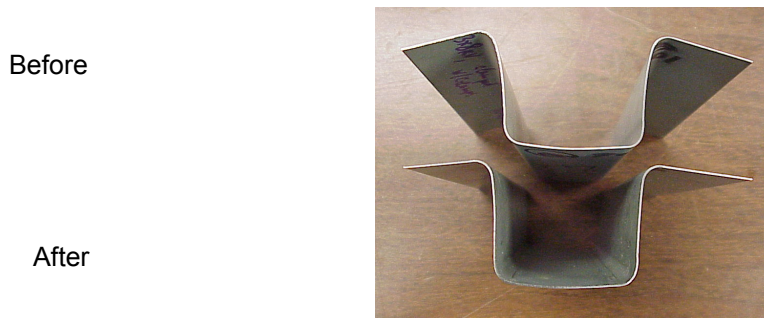
Figure 5: Comparison of U-channels before and after calibration
