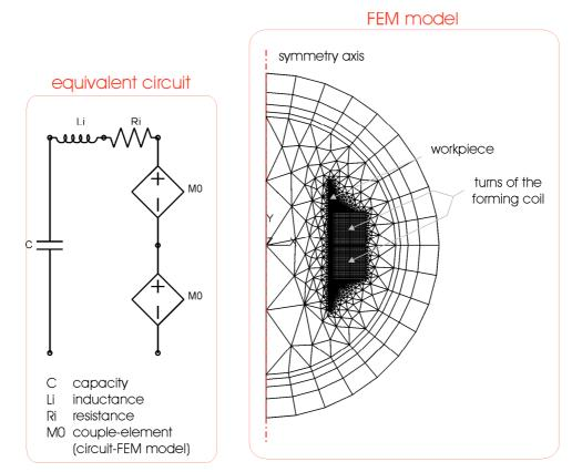
Figure 2: Coupling between equivalent circuit and FEM model
