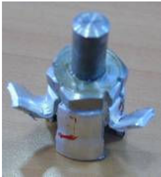
Figure 17: Peel test for Al3003-H12 to SS304
