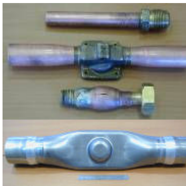
Figure 28: Cu/brass welds and Al/steel welds
