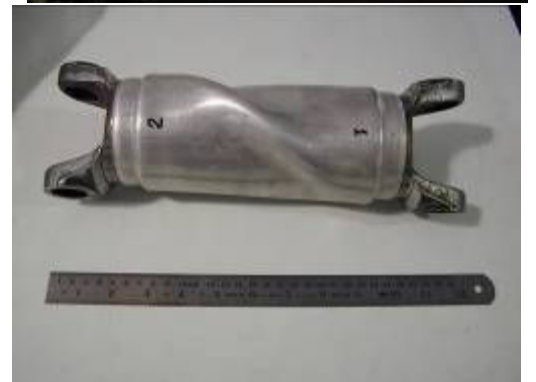
Figure 21: Torsion tested Al/Al 6061-T6 and Al/steel drive
