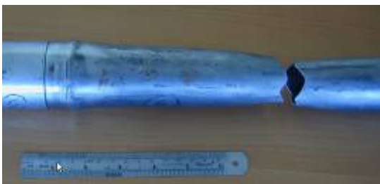
Figure 20: Tensile Test of welded 1020 steel tube
