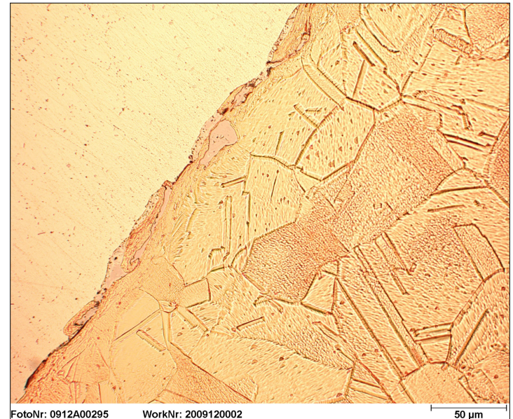
Detail MPW joint Al+Cu
