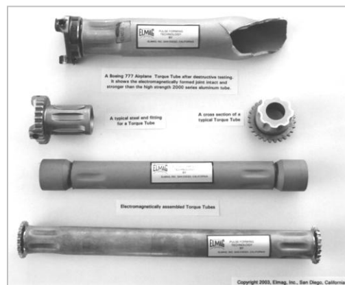
Figure 12: Aircraft Torque Tubes. These Tubes were anodized prior to forming. The cross section shows the intimate contact of the tube to the steel fitting.
