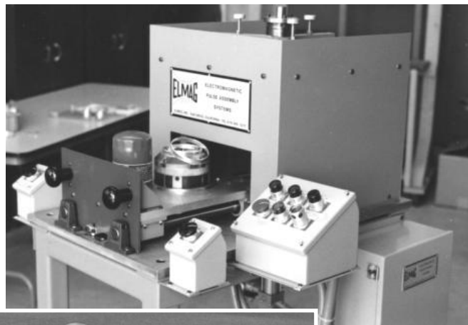
Figure 15: EMF system with work station to assemble EMI-proof connectors. It required a split coil to accommodate the geometry of 15 different sizes connectors and cables.
