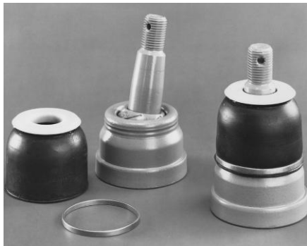
Figure 3: First industrial application used to shrink retaining rings onto neoprene boots. The above picture shows the ball joint before and after assembly.
