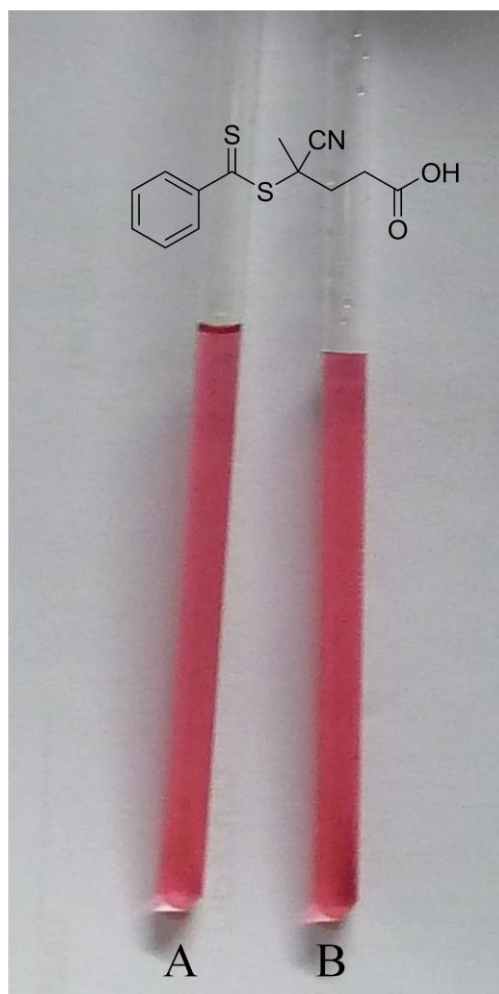
Figure 5.30 Photograph of a solution of RAFT agent in DMSO-d6, after treatment with aqueous HF solution (NH4HF2, 3M) (A) and before treatment (B).
