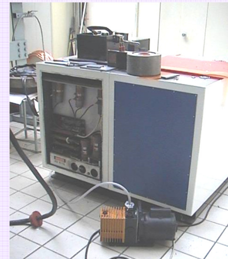
Magnetic Forming Generator
