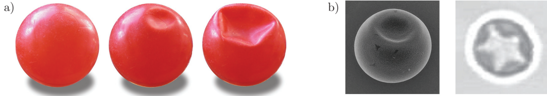
Figure 1.2.: The first and second buckling transition of a spherical shell can be observed on the macro- and microscale: a) a deflated plastic ball of diameter 5 cm, b) two microcapsules of diameter 2.5 μm (left, image taken from ref. [116]) and 5 μm (right, image taken from ref. [113]).
