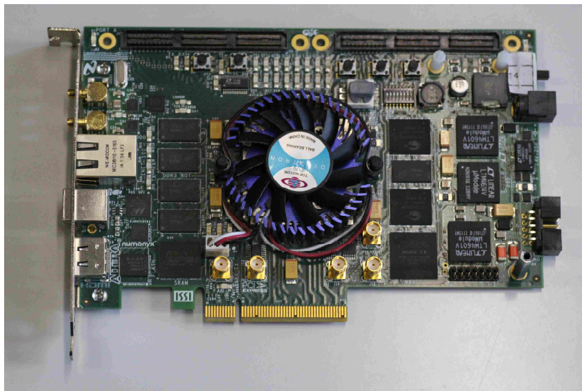
Figure 6.10: Picture of the used Stratix IV Development Kit DK-DEV-4SGX230N.
