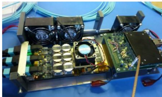
Figure 8.1: A picture of the MiniDAQ, consisting of an AMC40 prototype and a carrier board [49].
