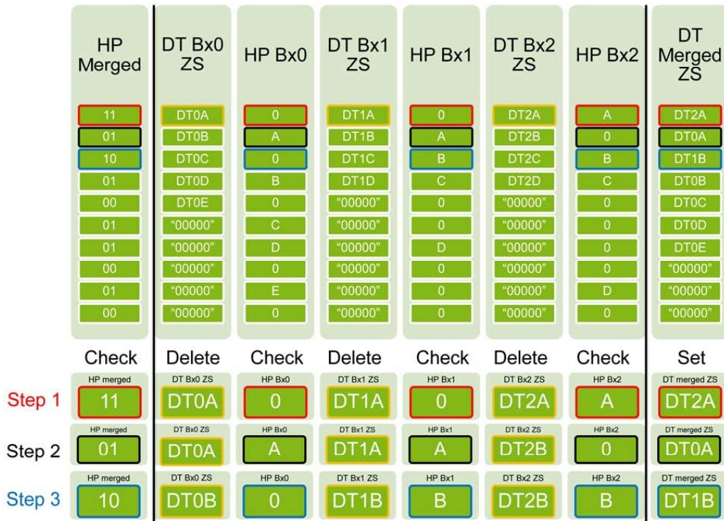
Figure 7.8: Illustration of an example for the step-by-step arranging method. In each step as marked in terms of colour (Step 1: red; Step 2: black; Step 3: blue) the hit pattern (HP) column is checked, indicated by the word "Check". In the drift time (DT) columns only the yellow marked part is checked and deleted if hit and thereby set to the merged DT column. Hereby ZS stands for zero suppressed.
