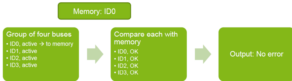
(a) All buses active and connected correctly: No error at output.
