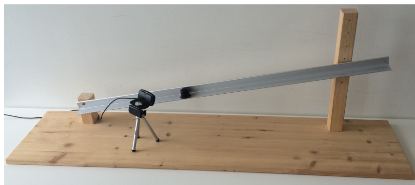
Figure 6.16.: Experimental setup of a capsule slide with mounted video camera.
