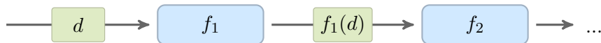
Figure 3.2.: Streaming functions f_i chained into a pipeline. The functions serve as the most atomic building blocks in the streams design approach.
