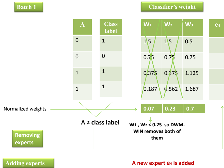
Figure 2.6: Overview of the steps of DWM-WIN in Batch 1: removing and adding of experts.
