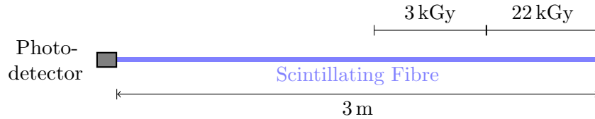
Figure 3.43: Simulated dose profile of fibre irradiation at CERN PS.
