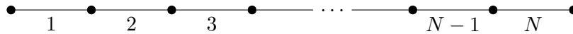
Figure 6.1.: Edges are streamed in ascending order with respect to their weights. The solution of the greedy algorithm is N whereas the optimal solution has weight at least \sum_{i=1}^{N/2} 2i \approx N^2/4 .
