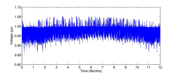
Figure D.2: Voltage at the end of the longest feeder in suburban grid new w/ appliances
