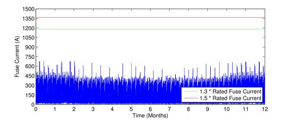
Figure 3.14: Current at transformer in suburban grid old w/ appliances and MV grid voltage fluctuations
