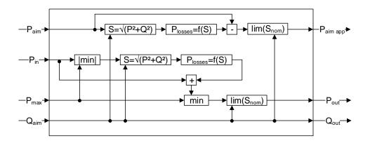
Figure 2.3: Block diagram of inverter model
