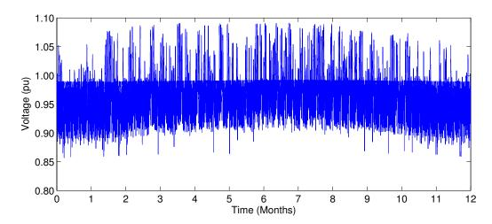
Figure 3.13: Voltage at the end of the longest feeder in suburban grid old w/ appliances and MV grid voltage fluctuations
