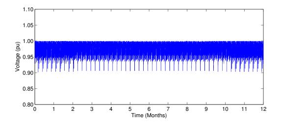
Figure D.20: Voltage at the end of the longest feeder in urban grid old w/ appliances
