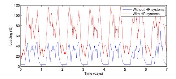
Figure C.2: Transformer loading characteristic of HP systems (suburban old grid)
