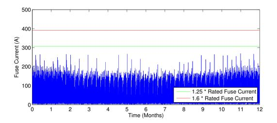
Figure 3.15: Current at beginning of considered feeder in suburban grid old w/ appliances and MV grid voltage fluctuations
