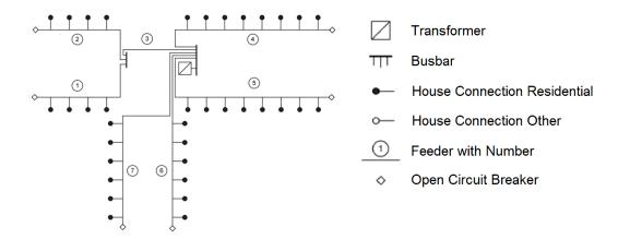
Figure 2.13: Grid topology of German urban low voltage grid [72]
