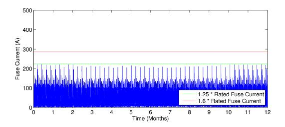
Figure D.24: Current at beginning of considered feeder in urban grid old w/ appliances and MV grid voltage fluctuations
