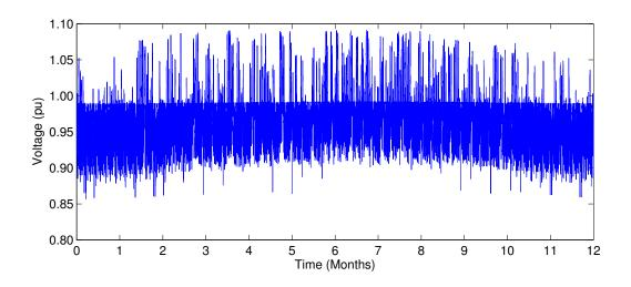
Figure D.10: Voltage at the end of the longest feeder in suburban grid old w/ appliances and MV grid voltage fluctuations
