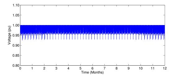
of the grid and the H0 profile do not completely match as can be seen in Figure B.1. The voltage level never rises above 1 pu as there are no generators connected.
