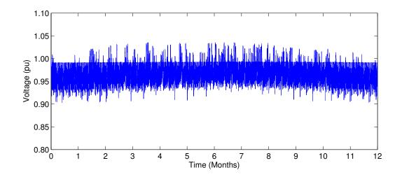
Figure D.15: Voltage at the end of the longest feeder in urban grid new w/o appliances including MV grid fluctuations
