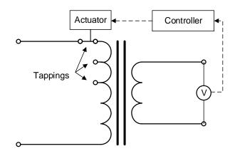
Figure 4.2: Schematic of OLTC principle
