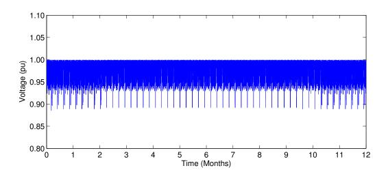
Figure D.7: Voltage at the end of the longest feeder in suburban grid old w/o appliances
