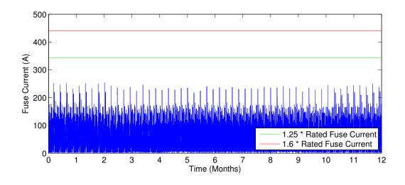
Figure 3.19: Current at beginning of considered feeder in urban grid new w/ appliances and MV grid voltage fluctuations
