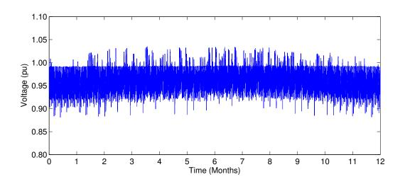
Figure D.22: Voltage at the end of the longest feeder in urban grid old w/ appliances and MV grid voltage fluctuations
