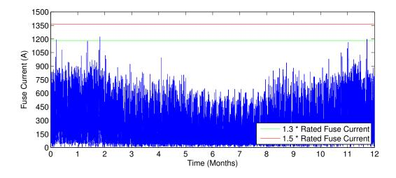
Figure 3.11: Current at transformer in suburban grid new w/ appliances and MV grid voltage fluctuations
