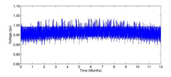
Figure 3.17: Voltage at the end of the longest feeder in urban grid new w/ appliances and MV grid voltage fluctuations
