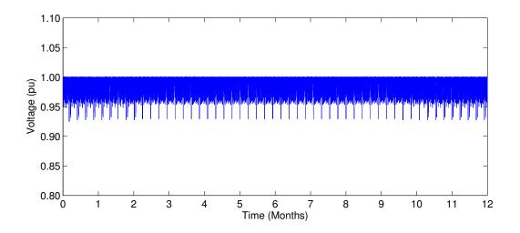
Figure D.1: Voltage at the end of the longest feeder in suburban grid new w/o appliances
