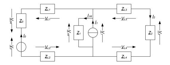
Figure 2.15: Equivalent circuit diagram of low voltage grid with generator and load
