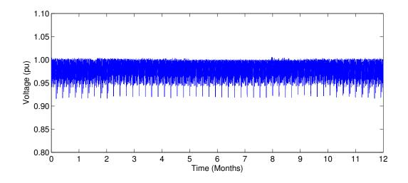
Figure D.14: Voltage at the end of the longest feeder in urban grid new w/ appliances
