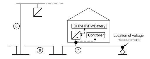
Figure 4.6: Schematic of end-user appliance based voltage control measures
