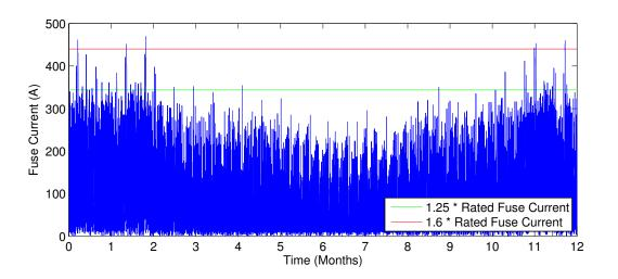
Figure D.6: Current at beginning of considered feeder in suburban grid new w/ appliances and MV grid voltage fluctuations
