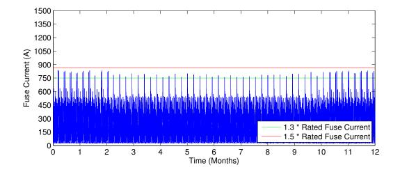
Figure D.23: Current at transformer in urban grid old w/ appliances and MV grid voltage fluctuations
