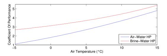
Figure 2.8: COP of 6kW<sub>th</sub> air-water and brine-water HP
