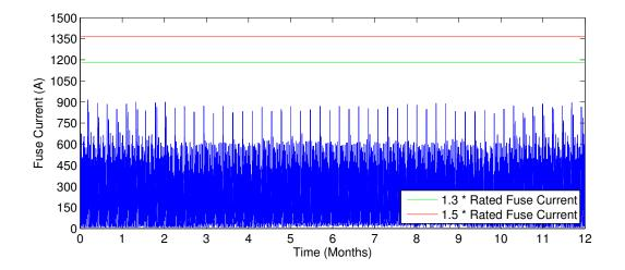
Figure D.17: Current at transformer in urban grid new w/ appliances and MV grid voltage fluctuations
