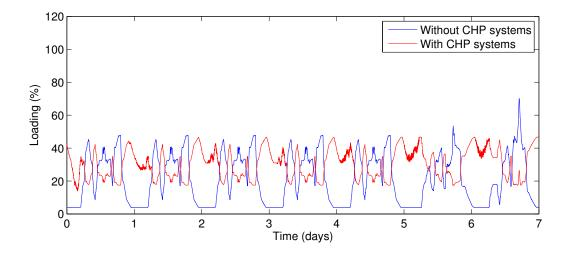
Figure C.1: Transformer loading characteristic of CHP systems (suburban old grid)
