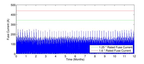
Figure D.18: Current at beginning of considered feeder in urban grid new w/ appliances and MV grid voltage fluctuations
