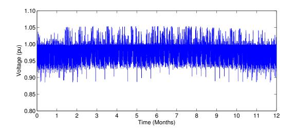
Figure D.8: Voltage at the end of the longest feeder in suburban grid old w/ appliances
