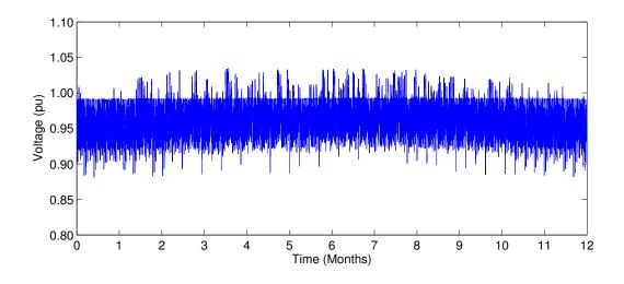
Figure 3.20: Voltage at the end of the longest feeder in urban grid old w/ appliances and MV grid voltage fluctuations
