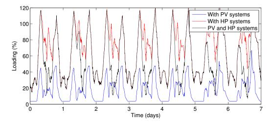
Figure C.5: Transformer loading characteristic of combined PV and HP systems (suburban old grid)
