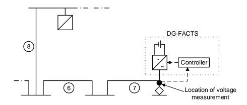
Figure 4.4: Schematic of DG-FACTS installation
