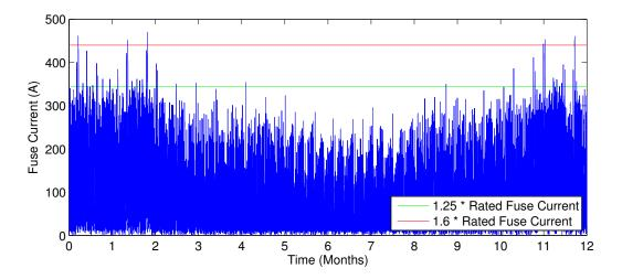
Figure 3.12: Current at beginning of considered feeder in suburban grid new w/ appliances and MV grid voltage fluctuations
