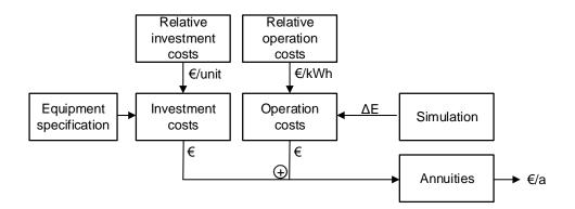
Figure 5.1: Schematic of cost calculation
