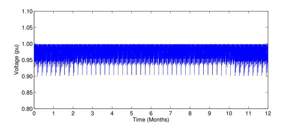
Figure D.19: Voltage at the end of the longest feeder in urban grid old w/o appliances
