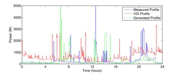
Figure 2.2: Examplary day profile of VDI 4655, Measured and Generated Profile
