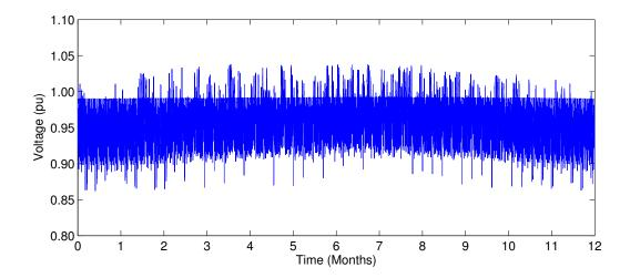
Figure D.9: Voltage at the end of the longest feeder in suburban grid old w/o appliances including MV grid fluctuations
