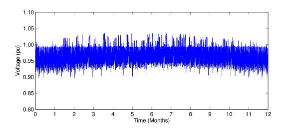
Figure D.16: Voltage at the end of the longest feeder in urban grid new w/ appliances and MV grid voltage fluctuations
