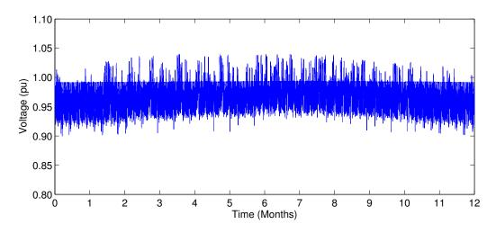
Figure D.3: Voltage at the end of the longest feeder in suburban grid new w/o appliances including MV grid fluctuations
