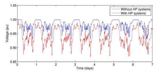
Figure 3.2: Voltage characteristic of HP systems at end of feeder 7 (suburban old grid)
