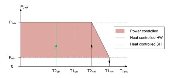
Figure 2.7: ICE and Stirling engine CHP hysteresis
