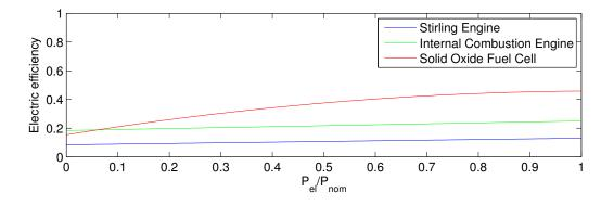
Figure 2.5: CHP electric efficiency
