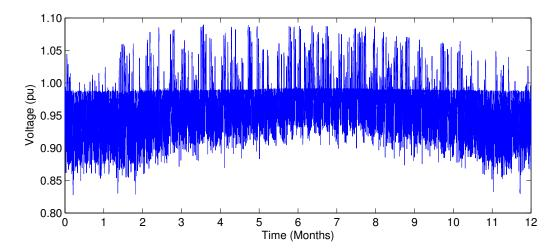
Figure D.4: Voltage at the end of the longest feeder in suburban grid new w/ appliances and MV grid voltage fluctuations
