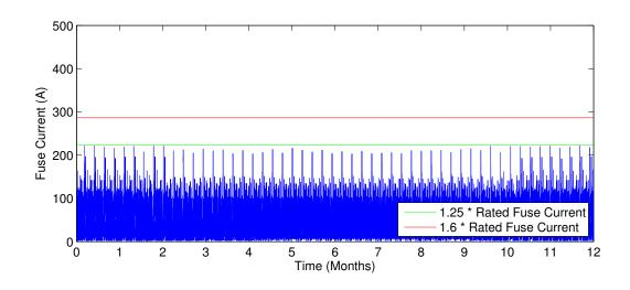
Figure 3.22: Current at beginning of considered feeder in urban grid old w/ appliances and MV grid voltage fluctuations
