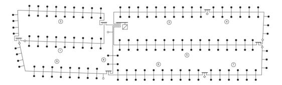
Figure 2.14: Grid topology of German suburban low voltage grid [72]
