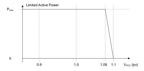
Figure 4.7: Proportional controller of measure active power control (APC)
