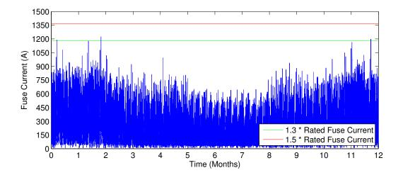
Figure D.5: Current at transformer in suburban grid new w/ appliances and MV grid voltage fluctuations
