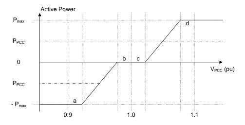
Figure 4.11: Proportional controller for active power of distributed storage for voltage control (stoV)
