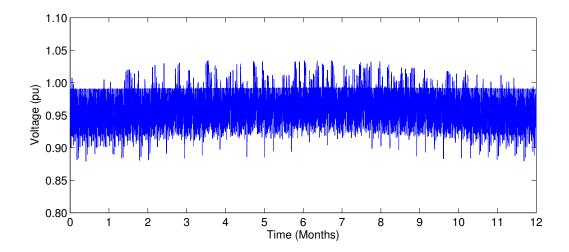
Figure D.21: Voltage at the end of the longest feeder in urban grid old w/o appliances including MV grid fluctuations
