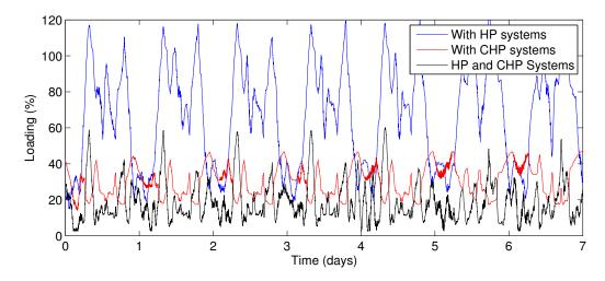
Figure C.4: Transformer loading characteristic of combined CHP and HP systems (suburban old grid)
