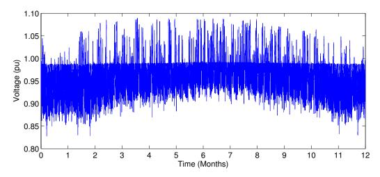
Figure 3.10: Voltage at the end of the longest feeder in suburban grid new w/ appliances and MV grid voltage fluctuations
