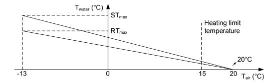
Figure 2.10: Heating characteristic to determine supply and return temperature
