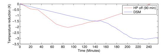
Figure 5.6: Temperature reduction due to SotA + DSM and HP shut down in reference scenario
