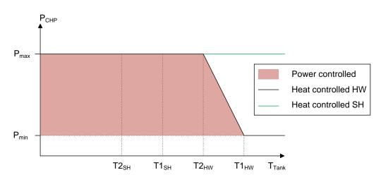
Figure 2.6: SOFC CHP controller
