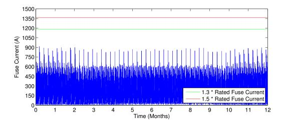
Figure 3.18: Current at transformer in urban grid new w/ appliances and MV grid voltage fluctuations
