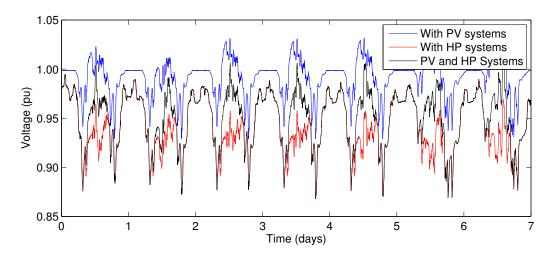
Figure 3.5: Voltage characteristic of combined PV and HP systems at end of feeder 7 (suburban old grid)
