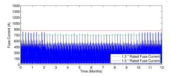
Figure 3.21: Current at transformer in urban grid old w/ appliances and MV grid voltage fluctuations
