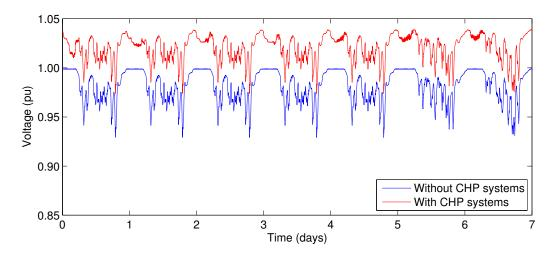
Figure 3.1: Voltage characteristic of CHP systems at end of feeder 7 (suburban old grid)
