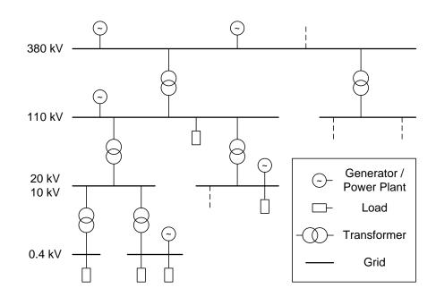
Figure 1.1: Overview on different grid voltage levels of the electricity system (Based on [4]).
