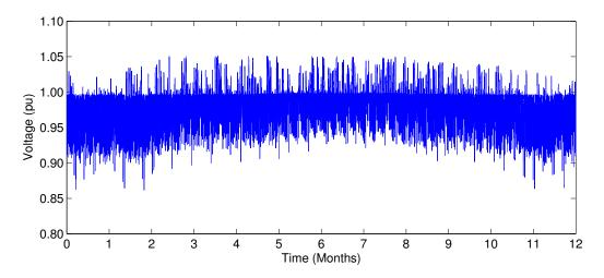
Figure 3.9: Voltage at the end of the longest feeder in suburban grid new w/ appliances
