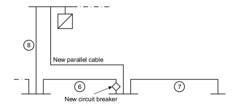
Figure 4.1: Connection schematic of additional parallel cable (Expansion)
