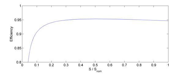
Figure 2.4: Efficiency characteristic of the inverter model
