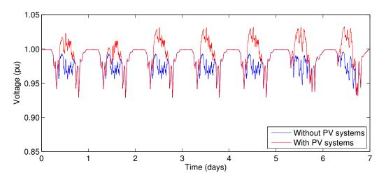
Figure 3.3: Voltage characteristic of PV systems at end of feeder 7 (suburban old grid)
