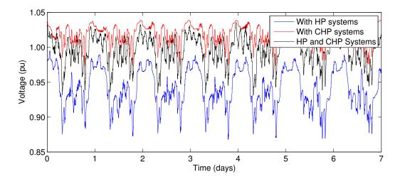
Figure 3.4: Voltage characteristic of combined CHP and HP systems at end of feeder 7 (suburban old grid)
