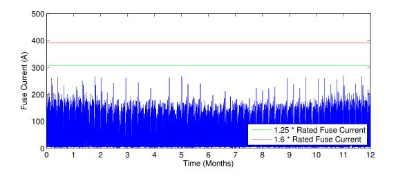
Figure D.12: Current at beginning of considered feeder in suburban grid old w/ appliances and MV grid voltage fluctuations
