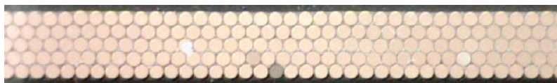
Figure 5.5: Cross section of a hand wound 2.5 m fibre mat on a wheel without a groove. [47]
