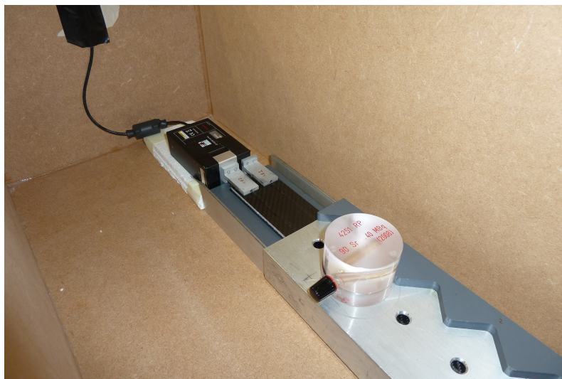
Figure A.7: Photograph of an in situ fibre module read out during a Technical Stop. The fibres are excited with a Strontium source and read out with an SiPM-usb-module.
