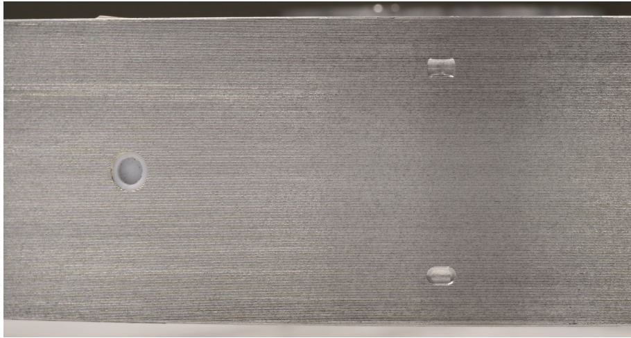
Figure 5.9: Different shaped prototype pin holes in the small Dortmund wheel. The cylindrical hole on the left is realised with a Teflon ® inlet to avoid the need of a release agent.
