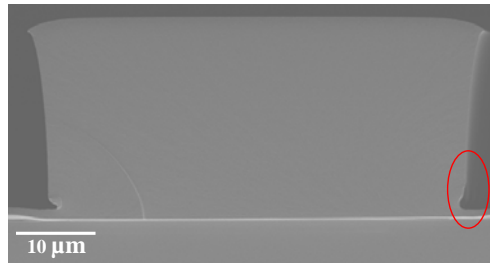
Fig. 7.3: SEM picture of Ormostamp resist (micro resist technology GmbH, Berlin, Germany) on nickel showing undercuts because of improper lithography process (courtesy of Victor Cadarso, PSI).
