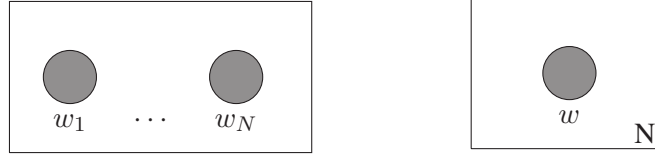
Figure 2.2.: Graphical representation of N independent random variables w . in the Plate notation Left: notation of N independence variables as shaded circular nodes, right: summarized notation of N independent variable as N times a single variable. For example, the MM with uni-gram LM can be graphically represented in such a way.
