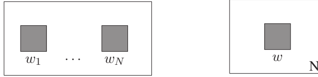
Figure 2.1.: Graphical representation of N independent variables w in the Plate notation. Left: notation of N independence variables as shaded rectangular nodes, right: summarized notation of N independent variable as N times a single variable. For example, the VSM with binary occurrences can be graphically represented in such a way.
