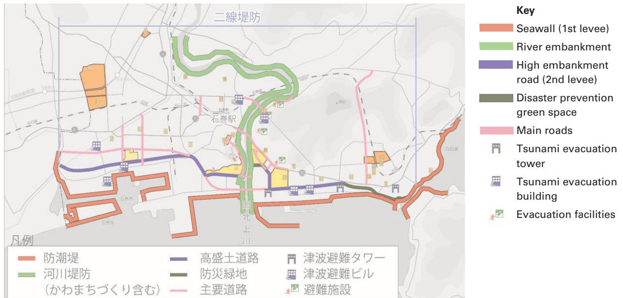
Illustration 63 | Map of planned protective infrastructure in Ishinomaki District (Ishinomaki City) | Ishinomaki City, 2016b, p. 32
