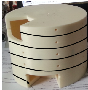
Figure 5.1: A 251 cm long fibre coiled in narrow groove and bonded with glue around a 3D printed cylinder. The fibre is highlighted in black.
