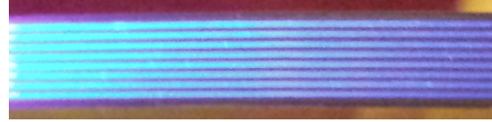
Figure 4.21: The fiber under test coiled around the plastic wheel. In this picture the fibre is excited with UV-light in order to improve visibility.
