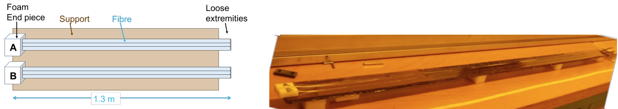
Figure 6.1: A sketch and a picture of the two bundles of 1.3 m long fibres glued on a light support. For clarity purposes, only 3 fibres per bundle are drawn in the sketch. In reality each bundle consists of a dozen of fibres.
