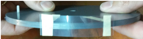
Figure 4.22: A picture of a transparent Gafchromic HD-810 dosimetric film fixed on the plastic wheel before irradiation.
