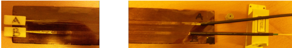
Figure 6.2: The fibres are loose at one extremity (right picture), while at the other extremity they are glued in a polystyrene foam end piece (left picture).
