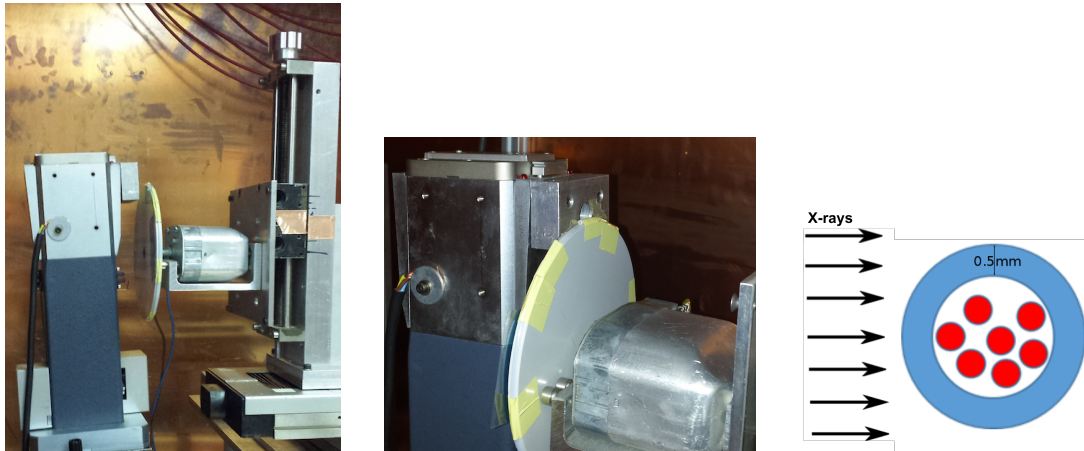
Figure 4.10: Pictures of the setup to irradiate a fibre sample with X-rays from a tube with Cu target. On the right a sketch of the cross-section of the teflon tube (in blue) containing the fibre sample (in red) is shown.
