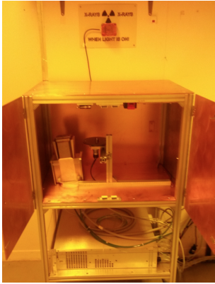
Figure 4.18: Custom-made shielding box containing the X-ray tube. The power supply is placed below the shielding box.
