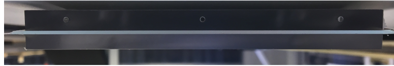
Fig. 7.26.: Photograph of a fibre mat cross section on the SiPM side. Three alignment holes are inserted in the upper SiPM end piece.
