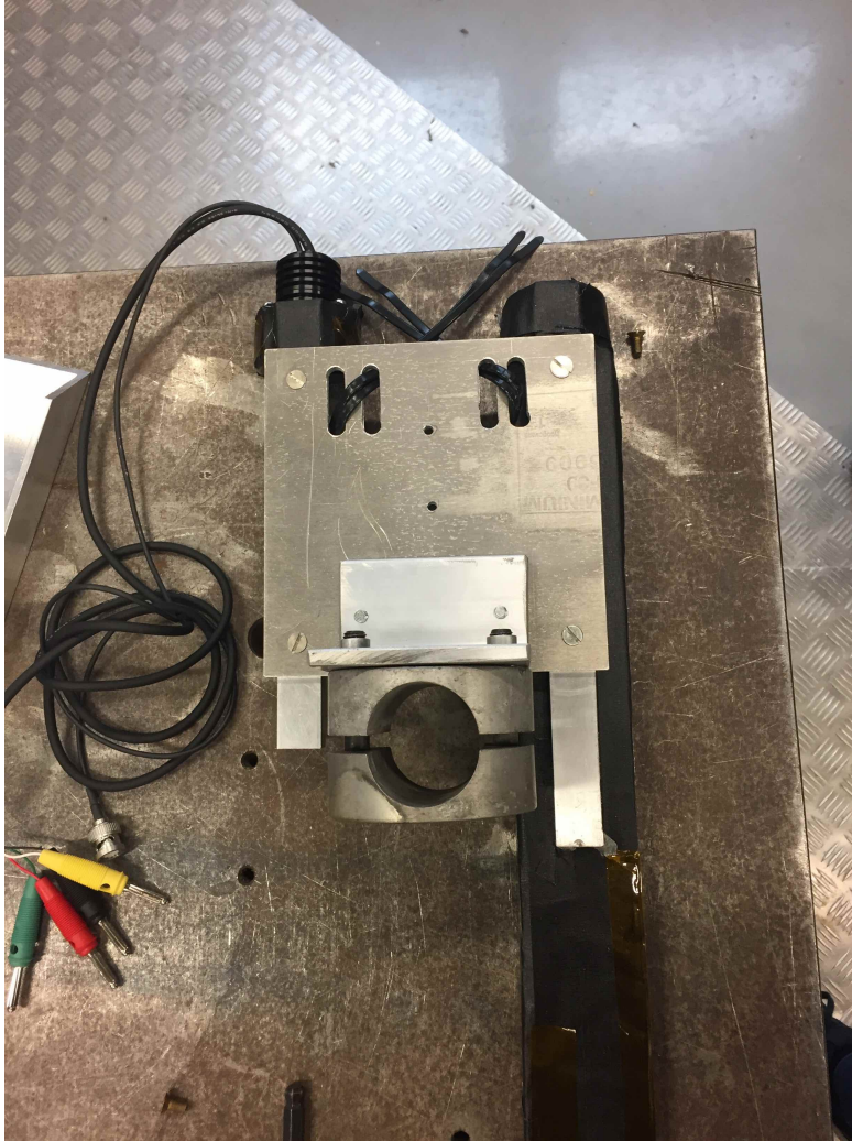
Fig. A.1.: Aluminium support, which holds the SiPMs and the fibre module. In addition it serves as mounting point for the installation in the cavern.
