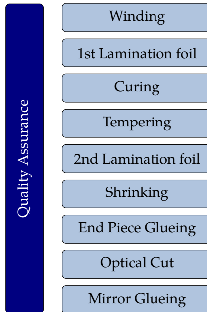
Fig. 5.2.: Necessary steps to produce a fibre mat. These steps are done in the Winding Centres, before the fibre mats get shipped to the Module Centres, where the side cuts are performed before assembling the detector module.
