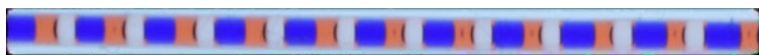
Figure 1. Gas-liquid-liquid slug flow with the doublet slug formed by the blue aqueous phase and the white gas phase separated by the red organic phase. The slug flow is flowing from right to left, with an average velocity of 30 \text{ mm s}^{-1} .
