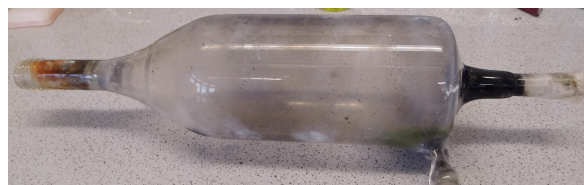
(b) Quartz glass reactor after ca. 1 hour bromination experiment 4
