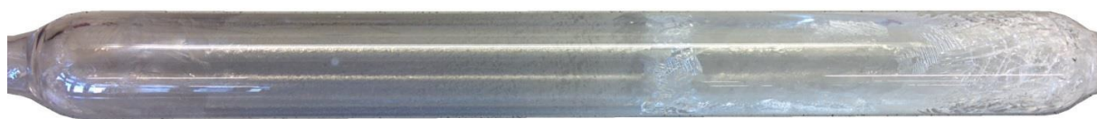
(a) Quartz glass reactor with solidification sacrificial wall after methane bromination experiment
