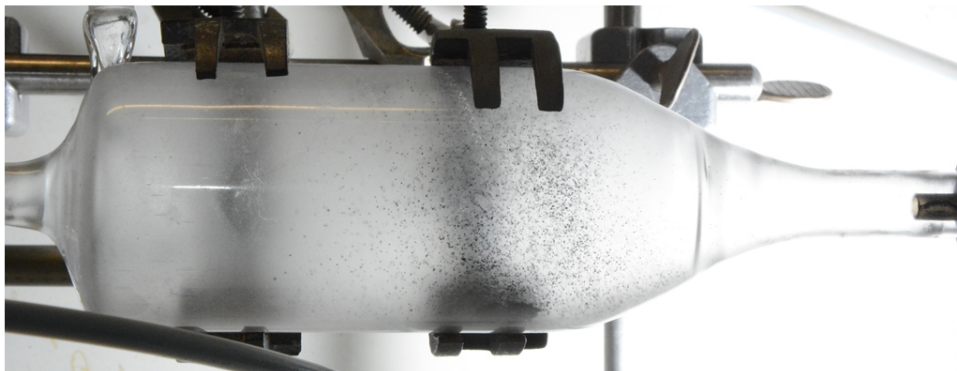
Figure B.12.: Carbon deposition on vortex flow reactor (co-current)
