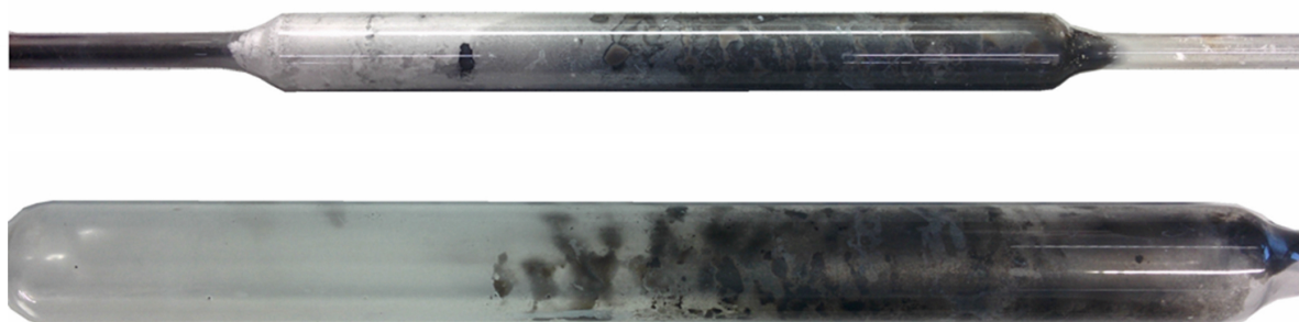
Figure 4.9.: Quartz glass tubular reactor with sacrificial wall after methane bromination experiment. Before (top) and after (bottom) dissolving sacrificial wall with water
