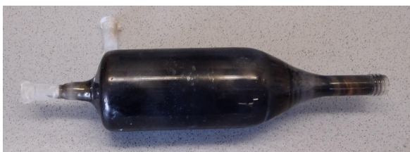
(a) Quartz glass reactor after ca. 1 hour bromination experiment 1
