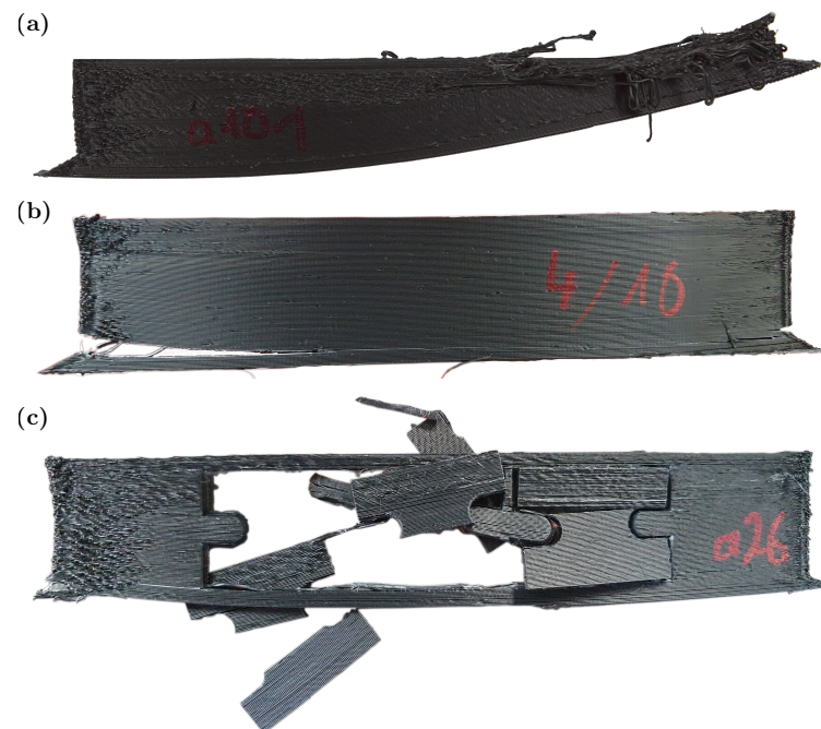
Figure 9. Examples of failed specimen fabrications and illustration of the consequences of extremely high in-process residual stresses in conventional processing of polypropylene. (a) Specimen with warping due to lack of print bed adhesion; (b) Cracked specimen as a result of in-process residual stresses; (c) Cracked specimen as a result of poor interlayer bonding.
