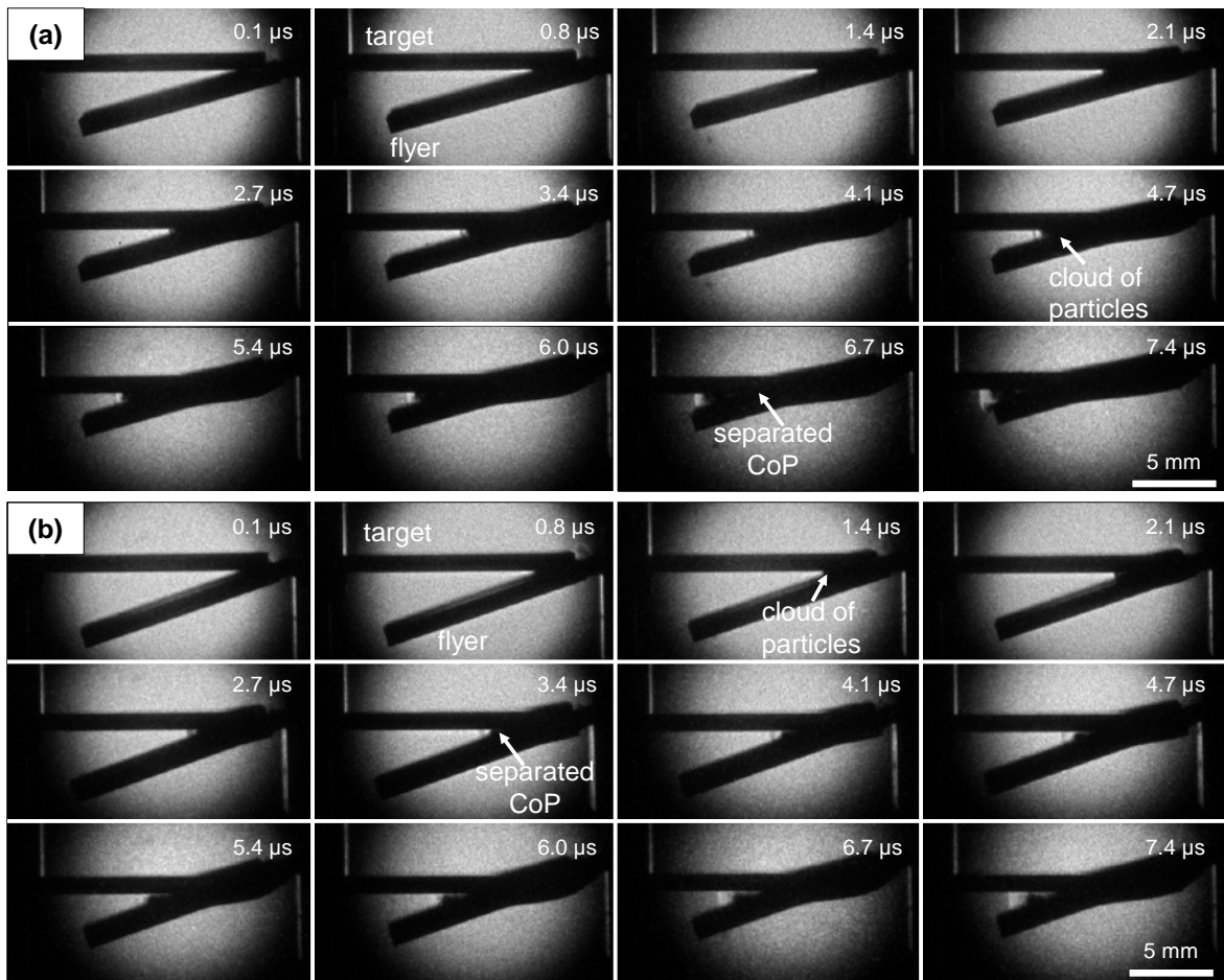
Figure 7: High Speed Imaging studies captured by the ML at the upper collision angle boundary at v_{imp} = 262 m/s. Each study consisted of three experiments taken at different delays. At \beta = 14.0^\circ a weld was achieved (a), at \beta = 16.2^\circ the samples were not welded (b). The accumulation of the CoP during the collision was higher in series (a) than in (b). A separation of the CoP from the apex of the joining gap starts earlier at (b) than at (a).
