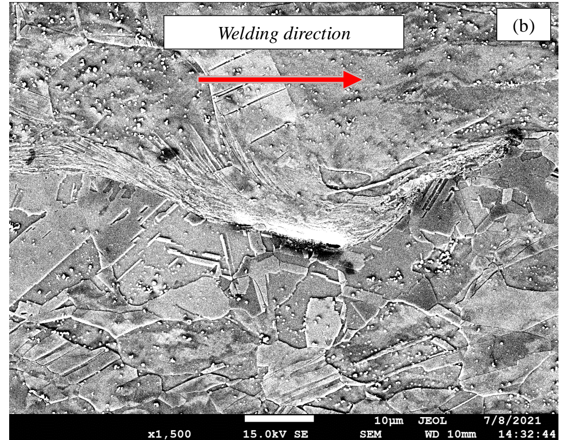
SEM images on JSM-7100F (Jeol) – (a) and (b) - Cu/Cu plates welded by MPW – Interface revealed after electro-polishing
