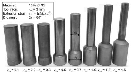
Figure A.2: Forward extruded 16MnCrS5 parts with various extrusion strains (adapted from Hering, 2020)
