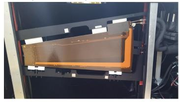
Figure 5.6: Petal core placed inside the PTM for thermal tests and held by a custommade frame.
