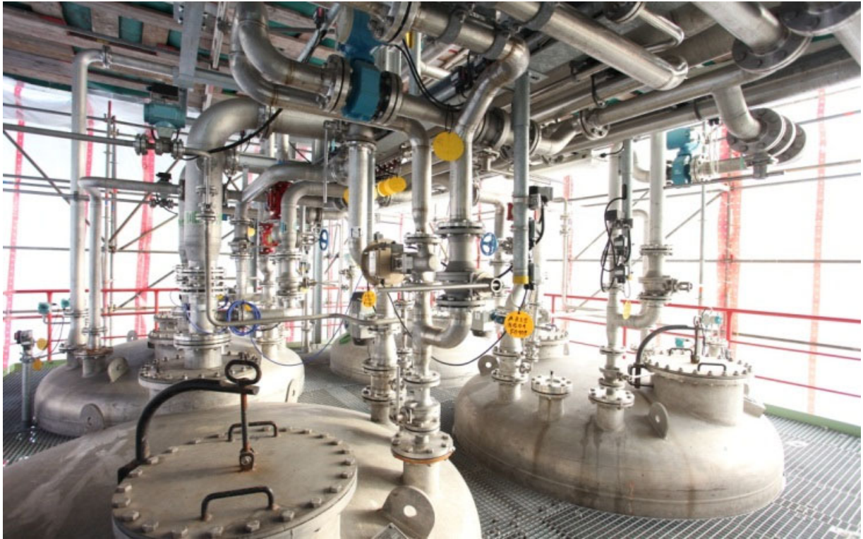
Fig. 2.12: Technical scale ozonation reactor (25 m 3 )
