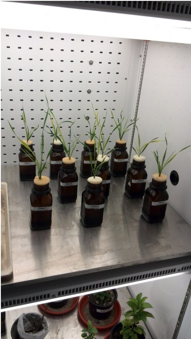
Figure 65. Experimental setup for root uptake of isotianil in wheat ( Triticum ) using a hydroponic system.
