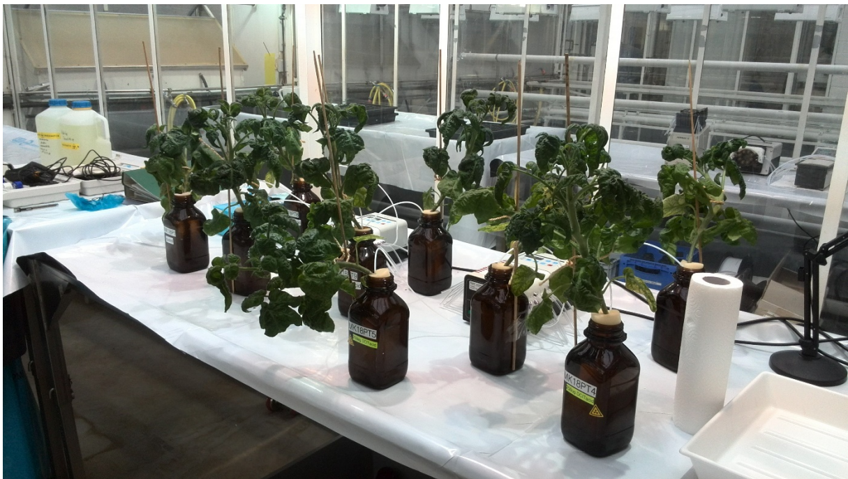
Figure 67. Experimental setup for root uptake of ^{14}\text{C} -labeled DCIT-acid in tomato ( Solanum lycopersicum ) using a hydroponic system.
