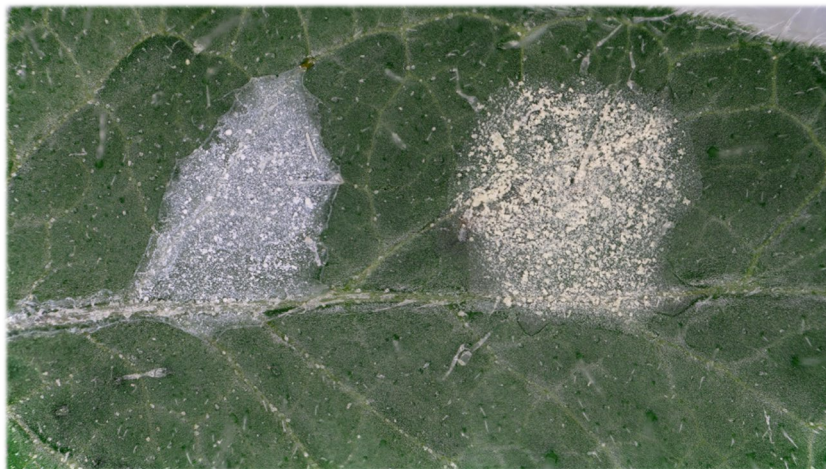
Figure 79. Optical image of tomato leaf ( Solanum lycopersicum ) with single droplet application of Propineb. Propineb as a WG70 formulation produces a homogenous layer on the tissue (left). Propineb mixed with HCCA produces a mesh of crystals on the tissue (right).
