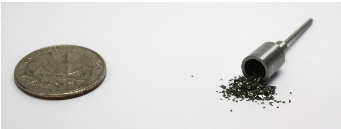
Figure 4.4: Illustration of a tungsten crucible used here for the evaporation of germanium pellets. A quarter dollar (left) serves as a scale.
