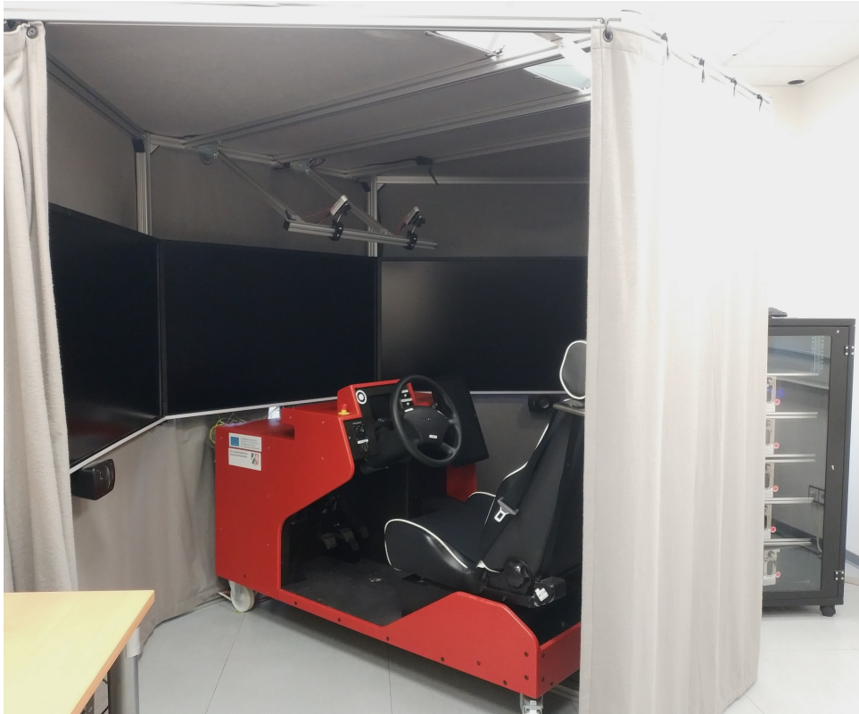
Figure A.2.: Driving simulator of the Institute of Control Theory and Systems Engineering at TU Dortmund University. It was used for conducting the driving simulator study.
