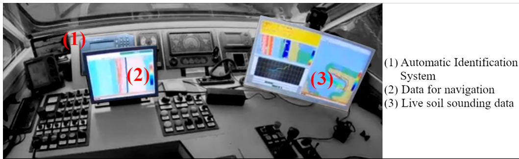
Fig. 7 Variety of information and monitors on a soil-sounding vessel
