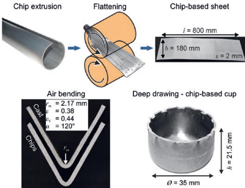
Production of chip-based sheets and further processing by bending and deep drawing
