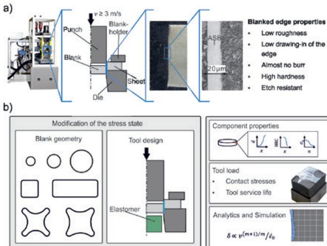
a) Schematic diagram of high-speed shear cutting, b) Focus of investigations
