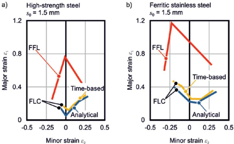
Representative FFL and FLC for a) high-strength steels and b) ferritic stainless steels
