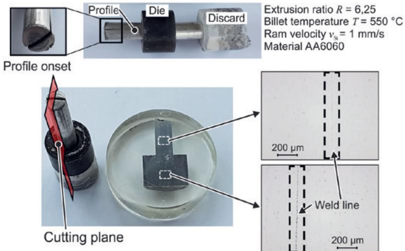
Profile extruded from half billets and detection of the weld line (optical microscope)
