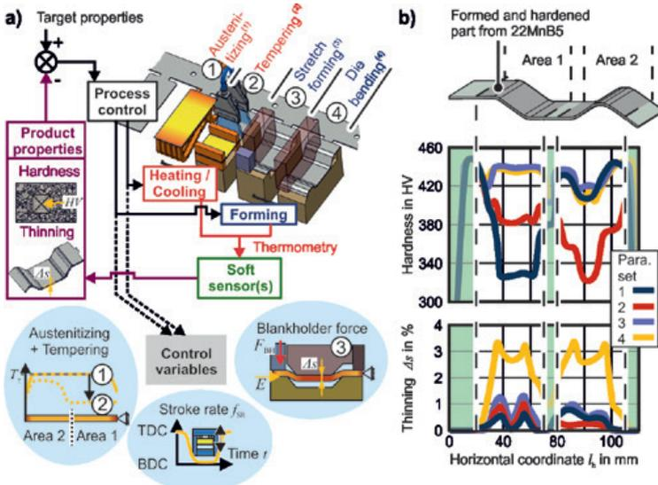
a) Control loop and tooling technology, b) Numerically determined hardness and thinning distribution for different control variable settings
