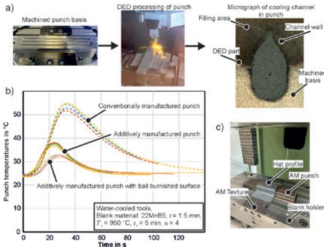
a) Manufacturing route of punch, b) Temperature measurement from: c) Hot stamping setup
