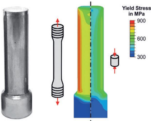
Yield Stress distribution in forward extruded rods, considering anisotropic hardening
