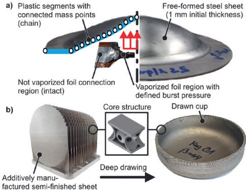
a) Selected topics: a) Vaporizing foil "chain model", b) Deep drawing of sheets with structured cores
