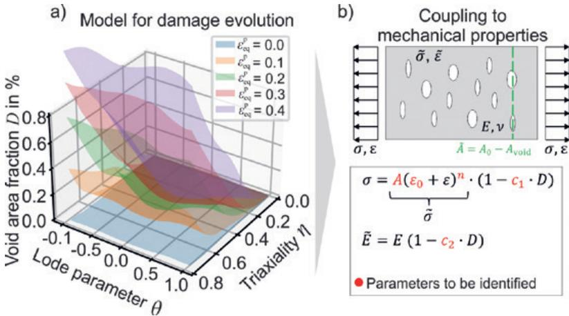
Development of a coupled damage model
