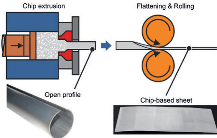
Process chain for the production of chip-based sheet
