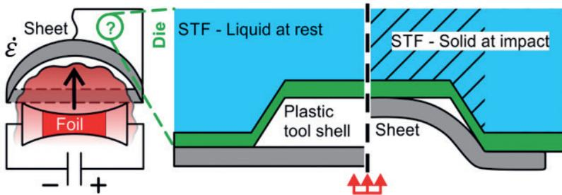
Schematic functioning of the tool concept for flexible high-speed sheet metal forming
