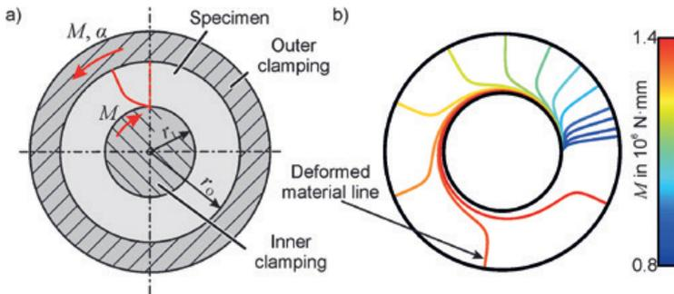
Principle sketch: Analytical model of the in-plane torsion test: a) Sketch of the specimen, b) Deformation of radial lines and the torque in the in-plane torsion test
