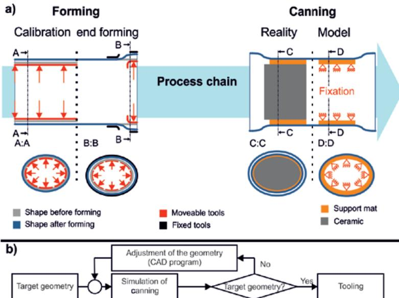
a) Process chain of catalyst, b) Optimization algorithm
