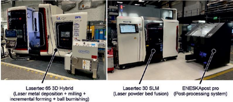
Figure 1: Machines for additive manufacturing based on metal powder at the IUL
