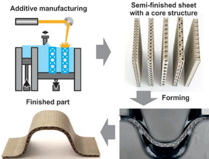
Process of additive manufacturing and subsequent forming
