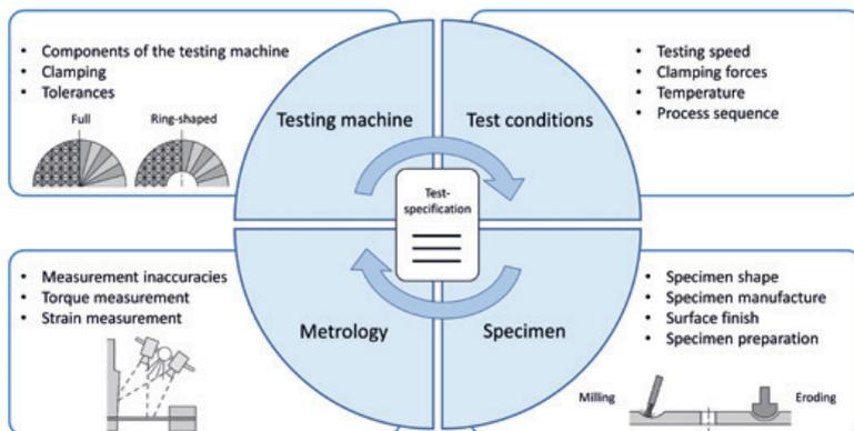
Overview of the four main fields of influences on the test results of the in-plane torsion test
