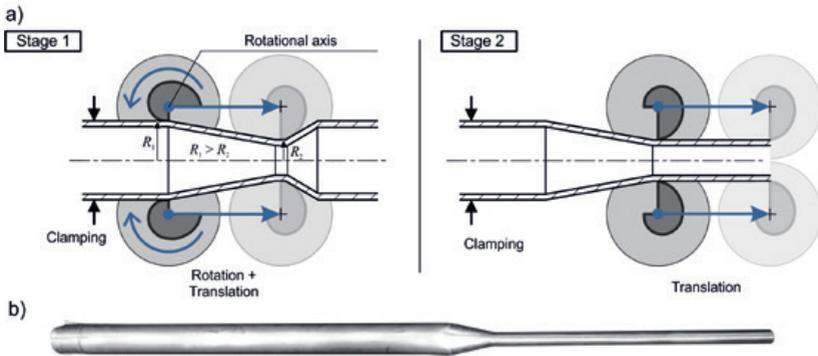
a) Combined roll gradation process, b) Formed workpiece
