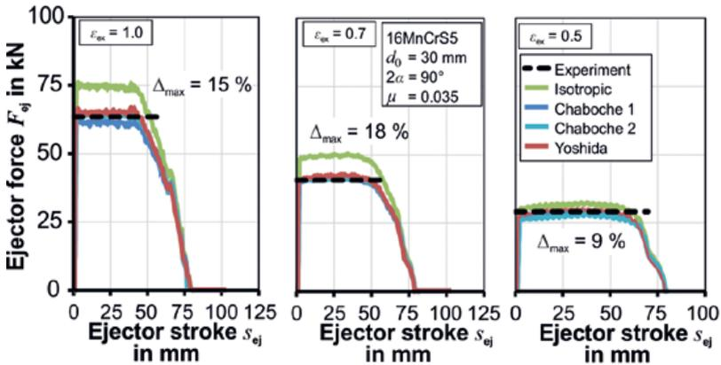
Numerically determined ejector forces in comparison with experiments
