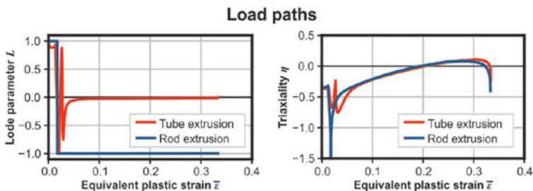
Experimental procedure to investigate lode angle dependency of damage evolution
