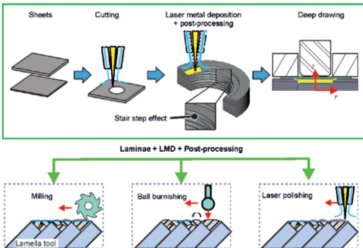
Figure 2: Process route for hybrid additive metal laminated tooling
