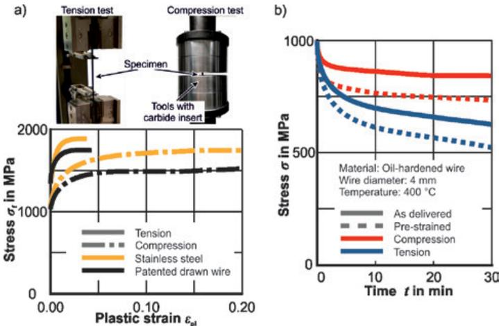
a) Flow curves from tension and compression tests, b) Stress relaxation behavior of oil hardened wire
