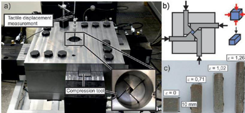
a) Structure of the equibiaxial compression test, b) Principle sketch, c) Formed tin specimen
