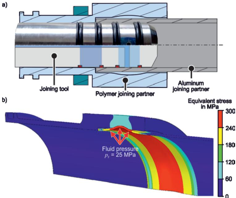
a) Initial situation of joining by hydraulic expansion, b) Numerical process design
