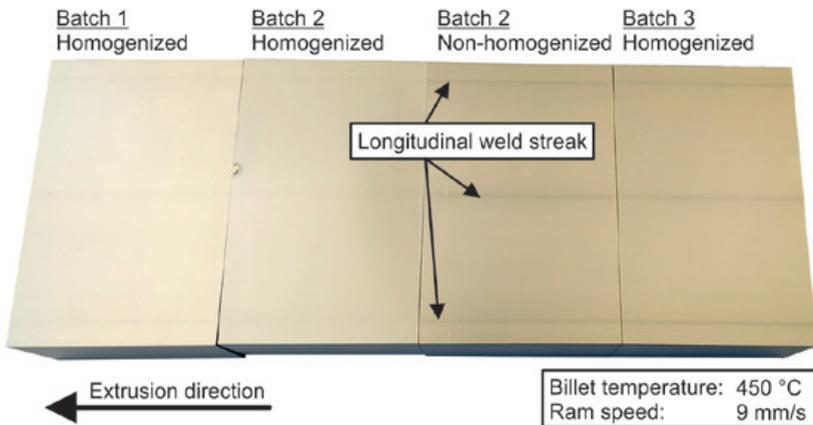
Influence of the pouring batch and homogenization of the billet on the weld streak formation
