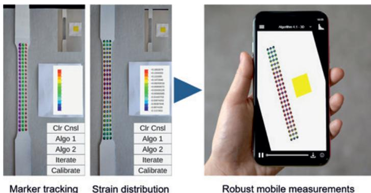
Concept of the mobile strain measurement application
