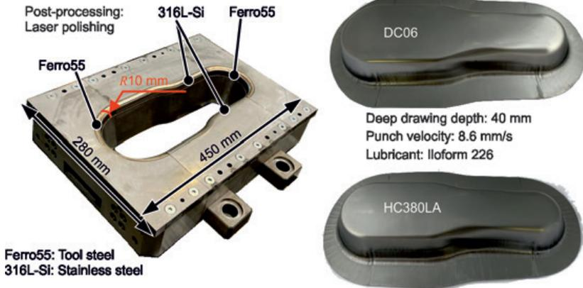
Manufactured hybrid deep drawing tool and parts
