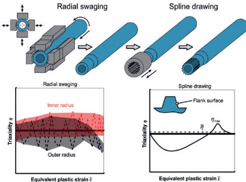
Oscillating load path in radial swaging and the load path on the flank surface of a tooth
