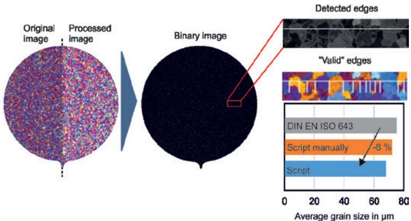
Schematic workflow of the automatic script to calculate grain size
