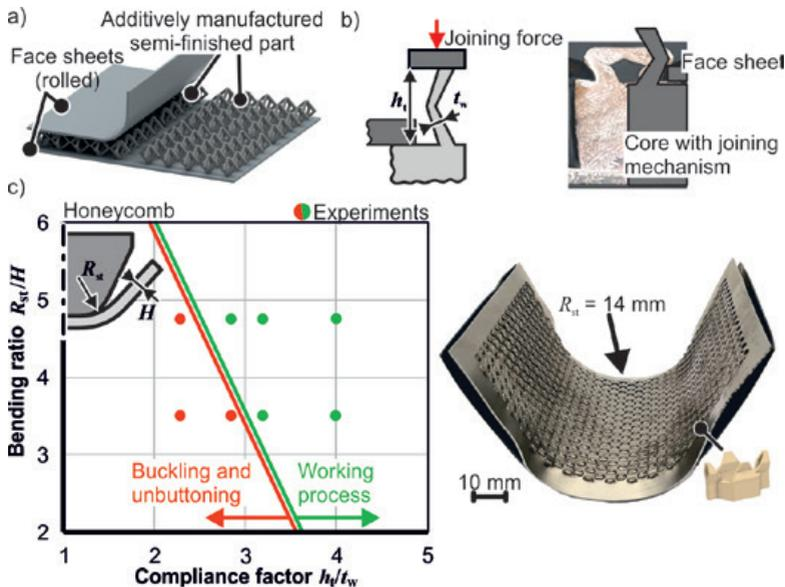
a) Large semi-finished sheet, b) Joining mechanism, c) Process window and bent component
