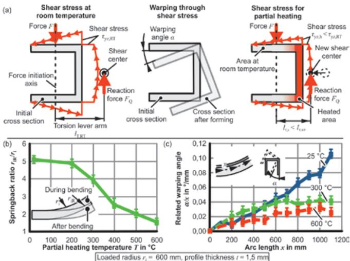
a) Principle of warping, b) springback, and c) warping for thickness bending with partial heating
