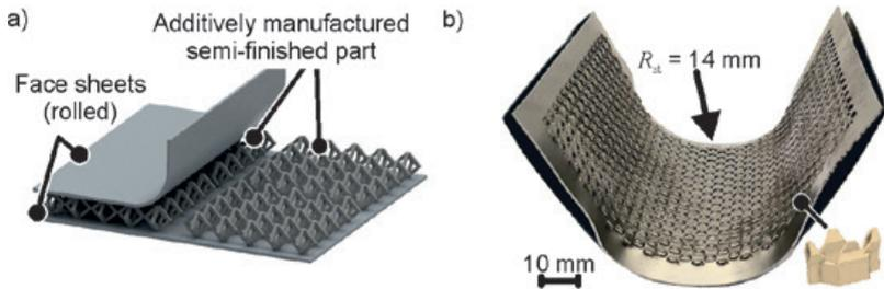
Figure 3: a) Principle of additively manufactured semi-finished part, b) Sandwich sheet after bending
