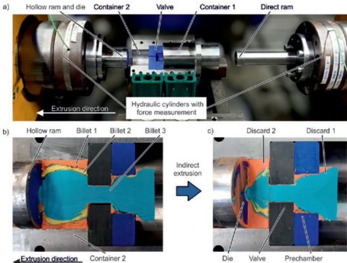
a) Experimental setup, b) and c) Material flow before and after indirect extrusion phase
