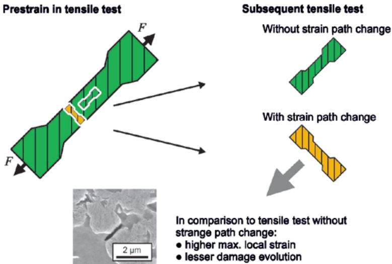
Multi-stage tensile tests on DP800
