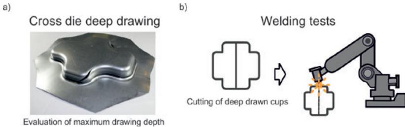
Investigation of green lubricants in a) Deep drawing and b) Subsequent welding
