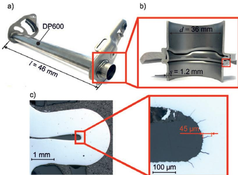
a) Height adjustment system, b) Cross section of the joints, c) Initial cracks at the inner bending radius
