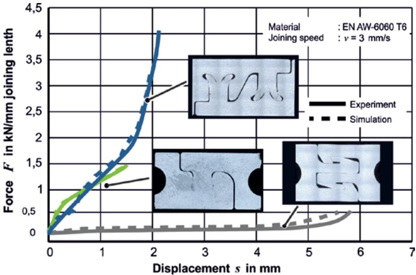
Longitudinal joining: comparison of joining simulation and experiments
