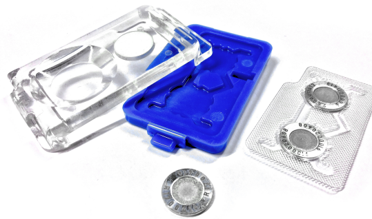
Figure 2.7: TL-DOS cassette with two blistered TL-DOS detectors to measure the irradiation quantities H_p(10) and H_p(0.07) (Image courtesy: MPA NRW).
