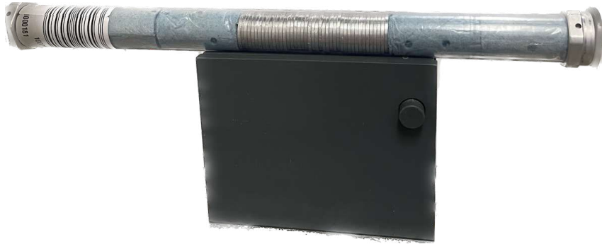
Figure 4.5: Partially filled detector magazine with 50 detectors on the holder. The detectors are centred within the magazine using cotton wool placeholders.
