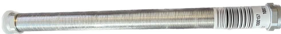
Figure 4.3: Filled detector magazine provided by the MPA NRW for storage and transportation of the TL-DOS detectors.
