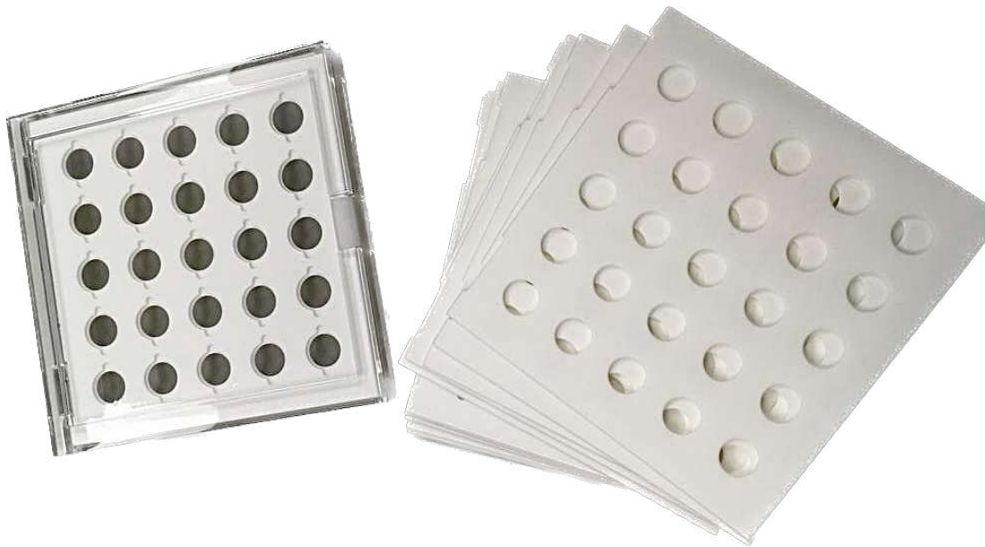
Figure 4.2: Irradiation frame provided by the MPA NRW for TL-DOS detector calibration.
