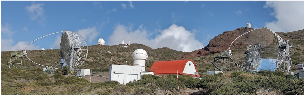
Figure 3.3: The MAGIC telescope system: MAGIC I (left) and MAGIC II (right). In between is the counting house: the computing, electronics, and operation center. The Light Detection and Ranging (LIDAR) tower (white) is mounted on the terrace of the counting house to protect the LIDAR from sunlight, rain, and wind.
