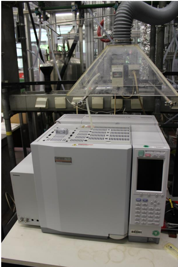
Figure 50: A fume extractor mounted above the gas chromatograph
