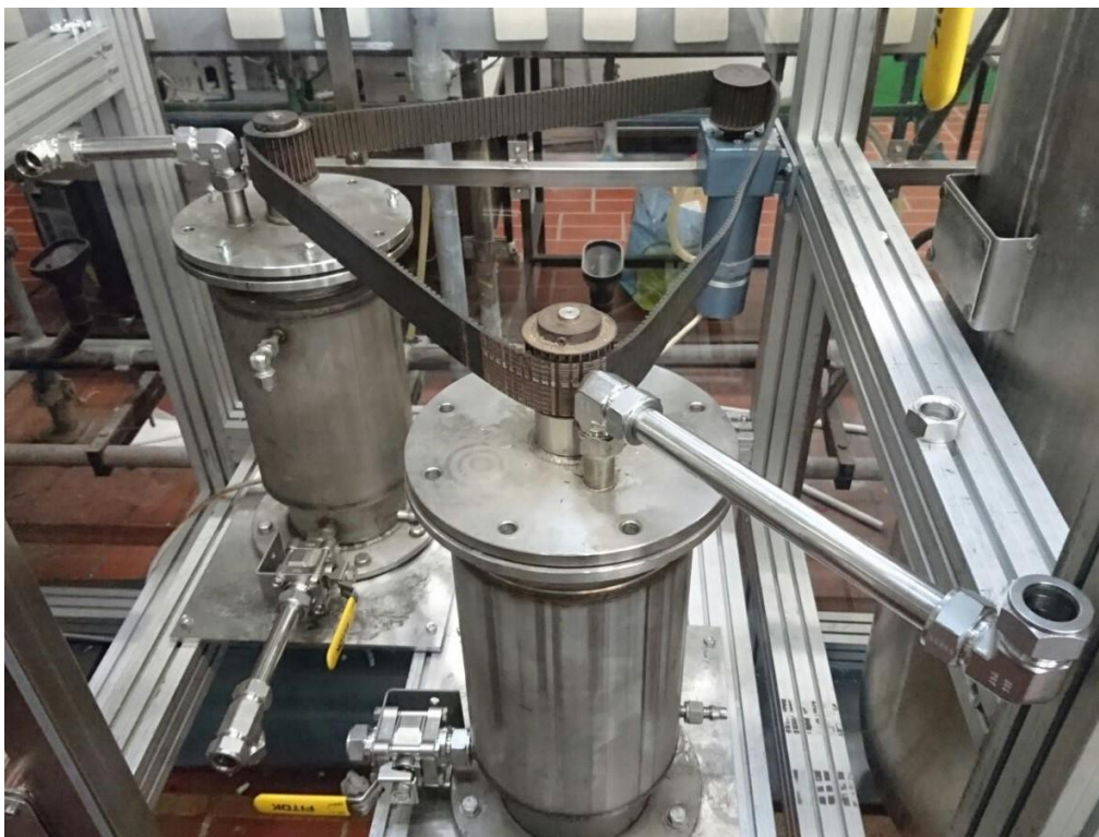
Figure 49: Scraped-wall desublimators for sulphur separation
