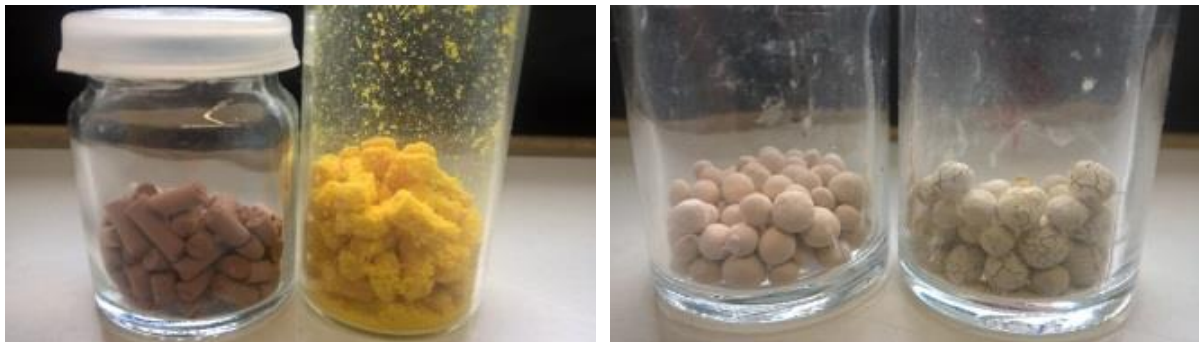
Figure 45: 3A Zeolite (right) and Zeolite AW-500 (left) before and after the exposure to HCl vapour and aq-HCl solution
