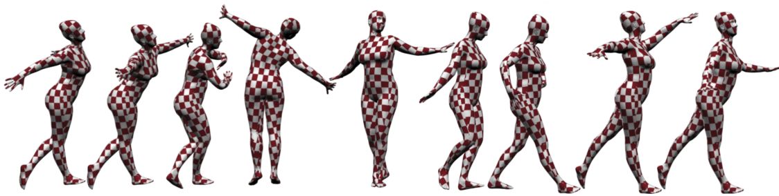
Figure 3.3.1: Example of a triangulated mesh representing a human from recordings of marker-based MoCap. Image taken from [LMB14].
