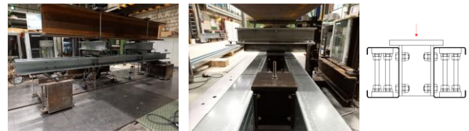
Figure 8 Test setup of the four-point bending tests and detail of the load application
