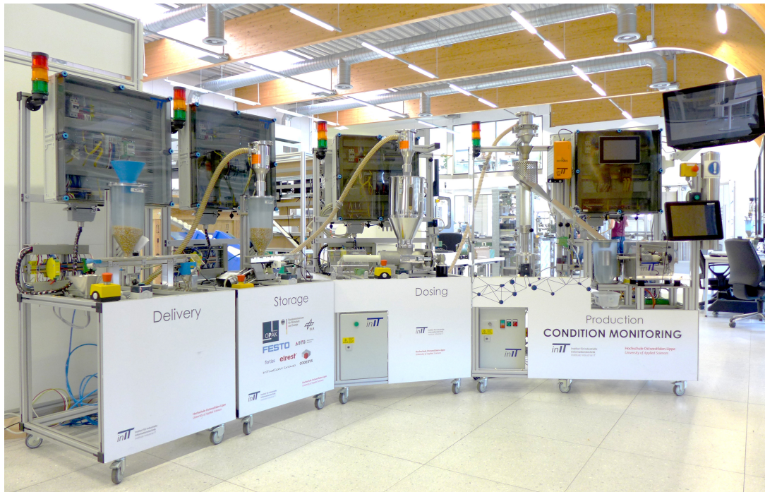
Figure 5.1: A modular and versatile production system to produce popcorn. The modules are equipped with compatible hardware interfaces, sensors, and actuators. The system can quickly be adapted if needed.
