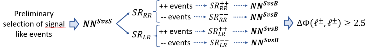
Figure 5.10: Schematic representation of the strategy followed to define the analysis SRs. First signal-like events are selected according to the criteria presented in Section 5.2.8. Events satisfying the preliminary selection requirements are employed to train the \text{NN}^{\text{SvsS}} to discriminate signal events originating from the RR or the two LR EFT operators. Four Signal Regions are defined based on the \text{NN}^{\text{SvsS}} output and on the charge of the same-sign leptons. A second \text{NN}^{\text{SvsB}} is trained over each SR to perform signal-background discrimination. A final selection requirement on \Delta\Phi(\ell^\pm, \ell^\pm) is used to complete the definition of the 4 analysis SRs.
