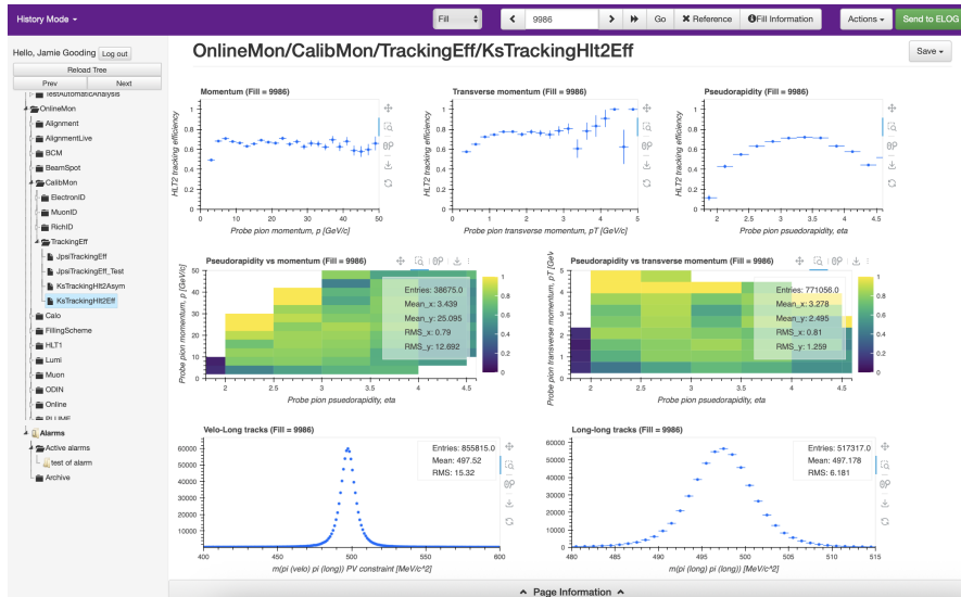
Figure 5.9: Monitoring web page for the CalibMon monitoring of K_S^0 \rightarrow \pi^+\pi^- for a single LHC fill in early 2024 data-taking.
